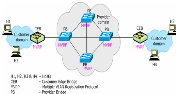
Figure 1: Example of a provider network supporting MVRP
